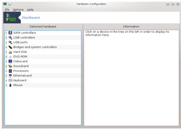
This tool<sup>11</sup> gives a general view of the hardware of your computer. When the tool is launched, it executes a job to look for every element of the hardware. For that, it uses the command ldetect which refers to a list of hardware in ldetect-lst package.
