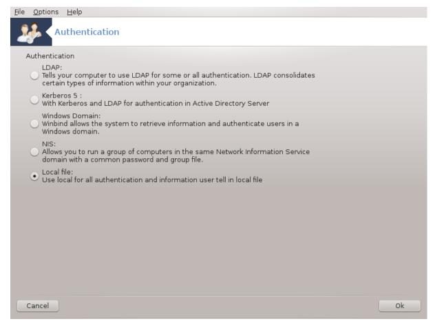
This  $tool^{26}$  enables you to modify the manner in which you can be recognized as user of the machine or on the net.
