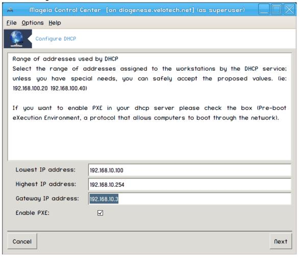
Select the beginning and ending IP addresses of the range of IPs you want the server to offer, along with the IP of the gateway machine connecting to some place outside the local network, hopefully close to the Internet, then click Next.
