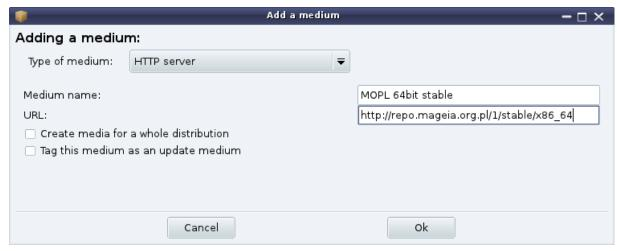
Select the medium type, find a smart name that well define the medium and give the URL (or the path, according to the medium type)
