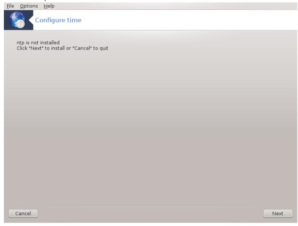
This tool<sup>9</sup> purpose is to set the time of your server synchronised with an external server. It isn't installed by default and you have to also install the drakwizard and drakwizard-base packages.
