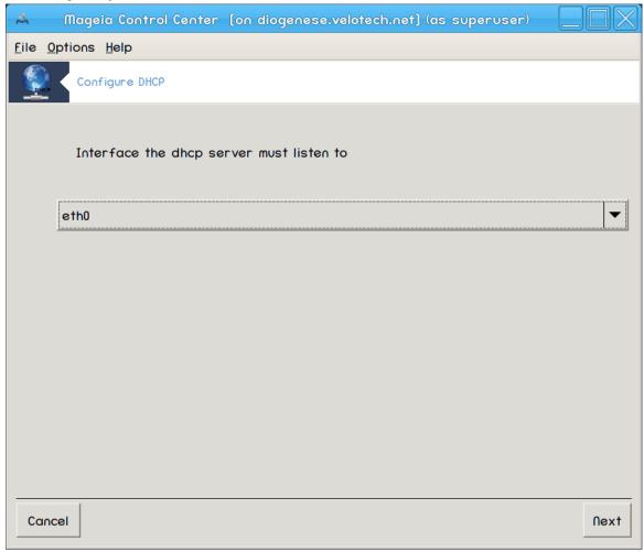
Choose the network interface, which is connected to the subnet, and for which DHCP will assign IP addresses, and then click Next.
