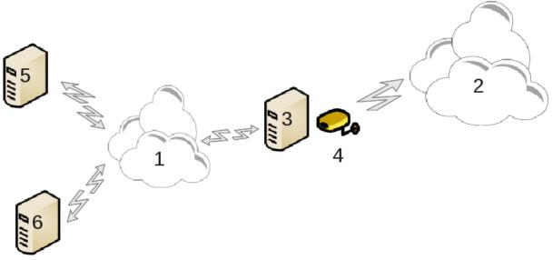
This is useful when you have a computer (3) which has Internet (2) access and is connected also to a local network (1). You can use computer (3) as a gateway to give that access to other workstations (5) and (6) in the local network (1). For this, the gateway must have two interfaces; the first one such as an ethernet card must be connected to the local network, and the second one (4) connected to the Internet (2).
