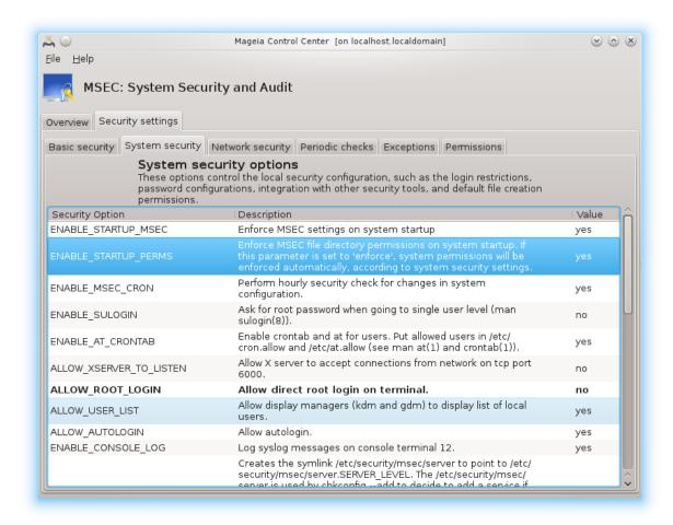
To modify an option, double click on it and a new window appears (see screenshot below). It displays the option name, a short description, the actual and default values, and a drop down list where the new value can be selected. Click on the OK button to validate the choice.
